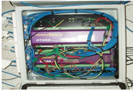
Figure 27: Cabling practice at the data logger box
