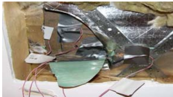
Figure 30: Cabling practice showing in-wall sensors, i.e., inside brick, outside building wrap, outside insulation, outside plasterboard surface and internal plasterboard surface
