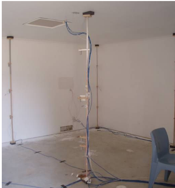
Figure 22: Sensors attached to the centre of room and edge of room poles
