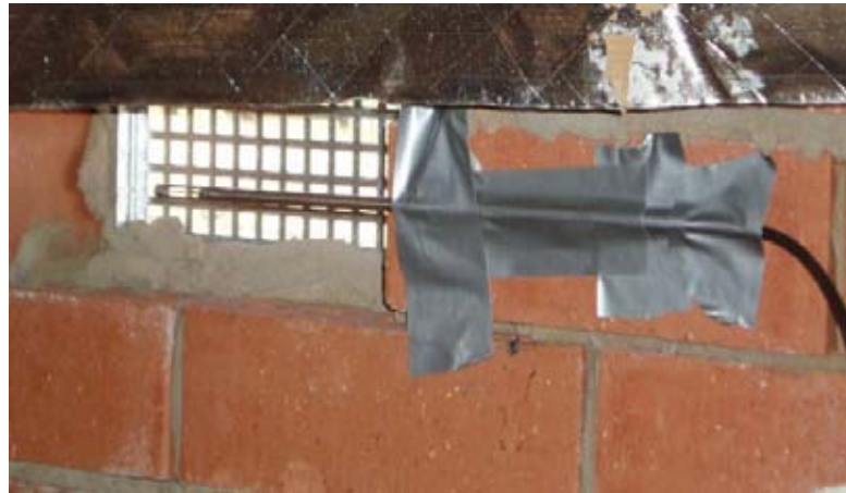
Figure 24: Hot Wire Air Speed Sensor at North Sub Floor Wall Vent
