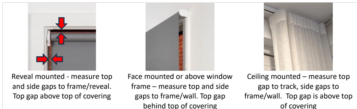
Figure 8.3 - Examples of edge gaps on different window coverings
