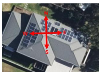
Figure 17.4 - Estimating array orientation
