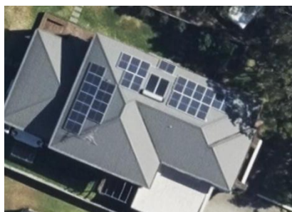
Figure 17.3 – Estimating system capacity - count the number of panels from a satellite image
