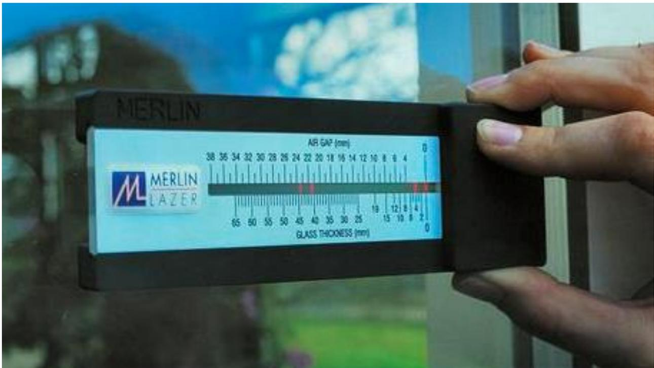
Fig. 6 – a commercial laser gauge to help identify the type of glazing installed within a window
