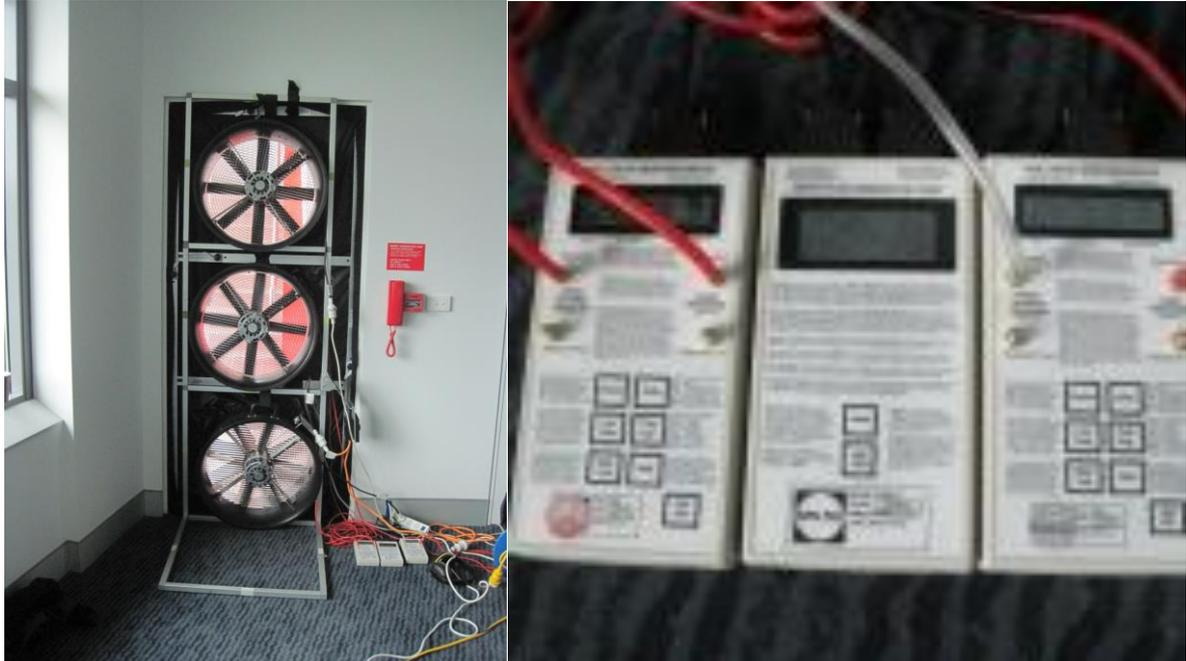
*Fig. 5 – BDT equipment (fans mounted to an external door and meters)*
